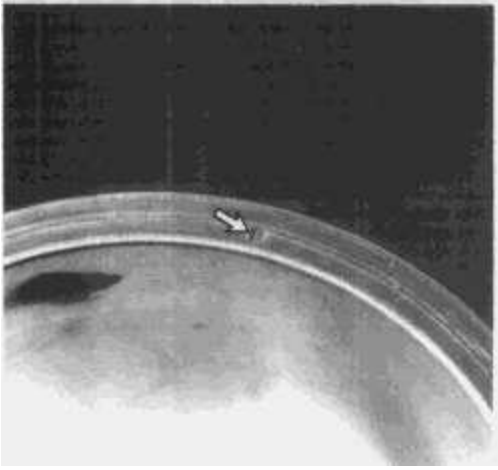
Damage to the fire dam. Use Again only if the damage is not extended completely across the fire dam and any burrs or sharp edges are removed.
