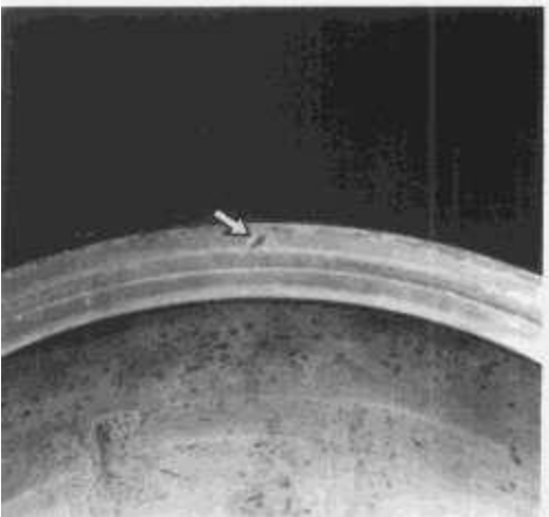
Damage in the gasket surface area. Do Not Use Again.
