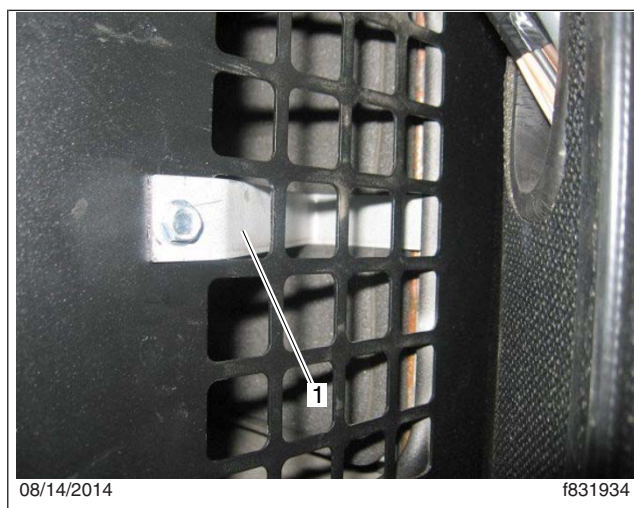
Fig. 5, Fresh-Air Door-Stop Bracket Installation
