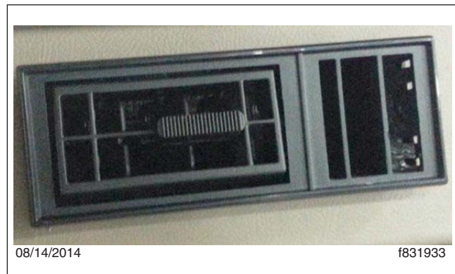
Fig. 4, New Right-Side Louver
