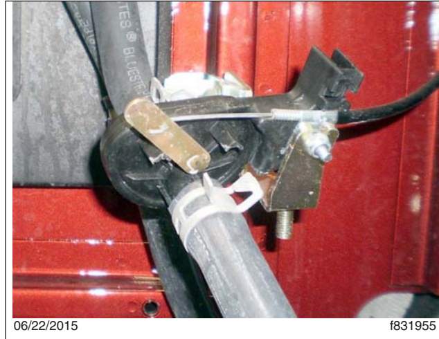
Fig. 13, Water-Valve Arm Resting on the Stop
