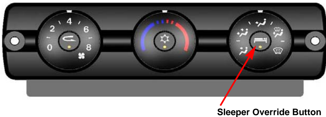
Figure 7-7: Cab Climate Control Panel in a Sleeper Cab
