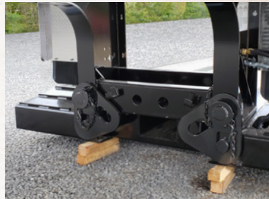
Figure 8 plate (also known as "lock rings" or "swinging tear-drops") features options for 50" or 52" loaded fifth wheel height.
