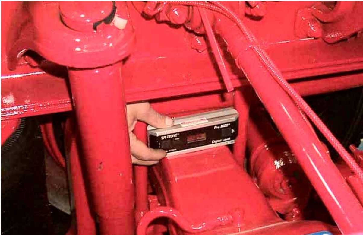
Figure 9 Illustration of Using an Inclinometer to Determine Forward Rear Axle Angle
