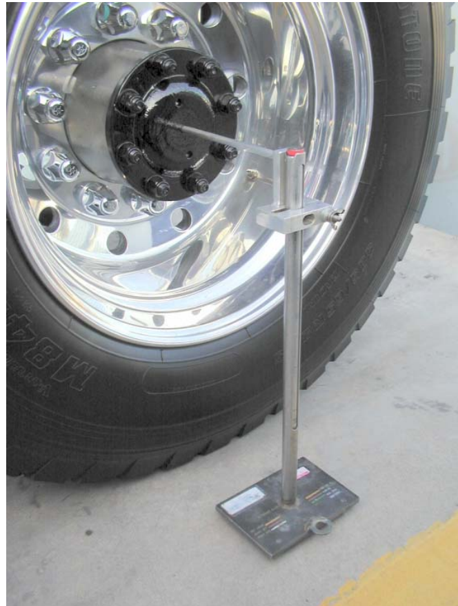
Figure 2 Illustration of Aligning The Pointer of a Ride Height Gauge
