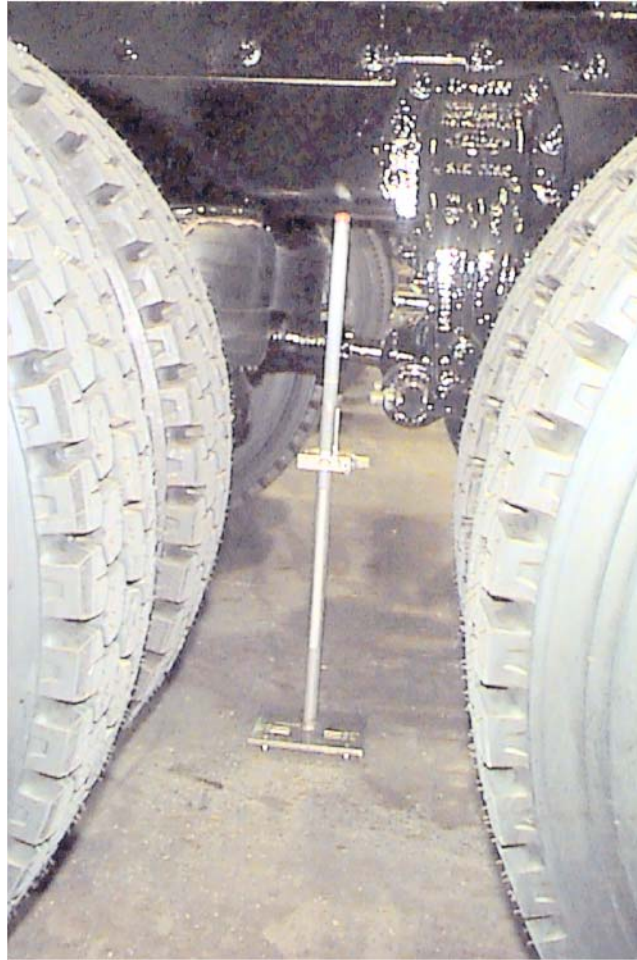
Figure 3 Illustration of Measuring The Ride Height on a Tandem Suspension
