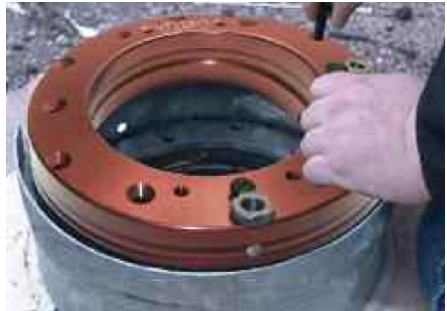
The drill fixture ring is shown here installed on an extension and is elevated for illustration purposes only.
