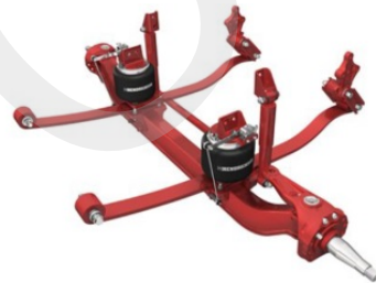
Original Manufacturer Equipment (Leaf/Air Primary Suspension)
