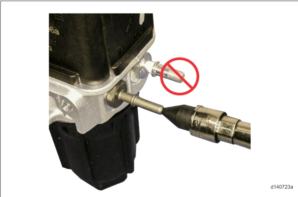
19. Connect all DEF lines and electrical connections. [Go to step 20.](#)
